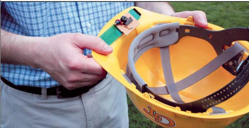
Two academics have developed a system that uses ambient radio waves, rather than batteries, to generate energy for mobile devices. They have built the system into a prototype hard hat that uses the energy to detect if wearers get too close to potentially dangerous equipment on a work site and to then sound a warning.
